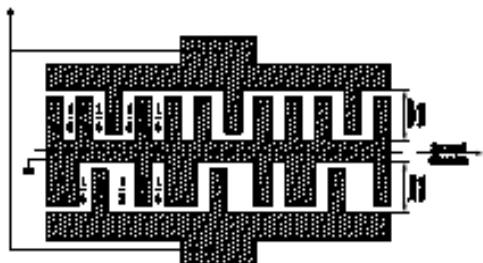
Figure 21 Waveguide SPUDT, reprinted from [42]. The SPUDT is achieved by using the transverse wave coupling between tracks.
