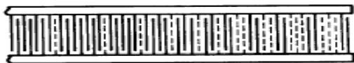
Figure 9 Example of a withdrawal weighted IDT transducer, reprinted from [22]. The dotted lines represent removed or “withdrawn” electrodes.
